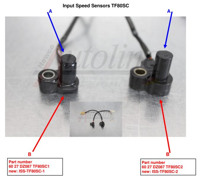
Both sensors have a white 2-pole/prong-connector with a red and a white cable. Length of cable and type of connector are the same
